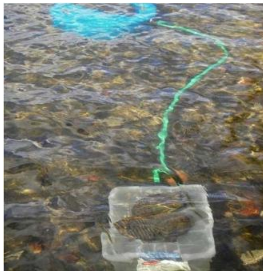
Figure 4: Seepage Meter (Blue Cylinder) Attached to Measuring Bag (Protected From Waves and Wind by the Clear Plastic Case)
